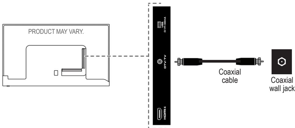
1. Connect a coaxial cable (not included) to your cable/satellite box.
