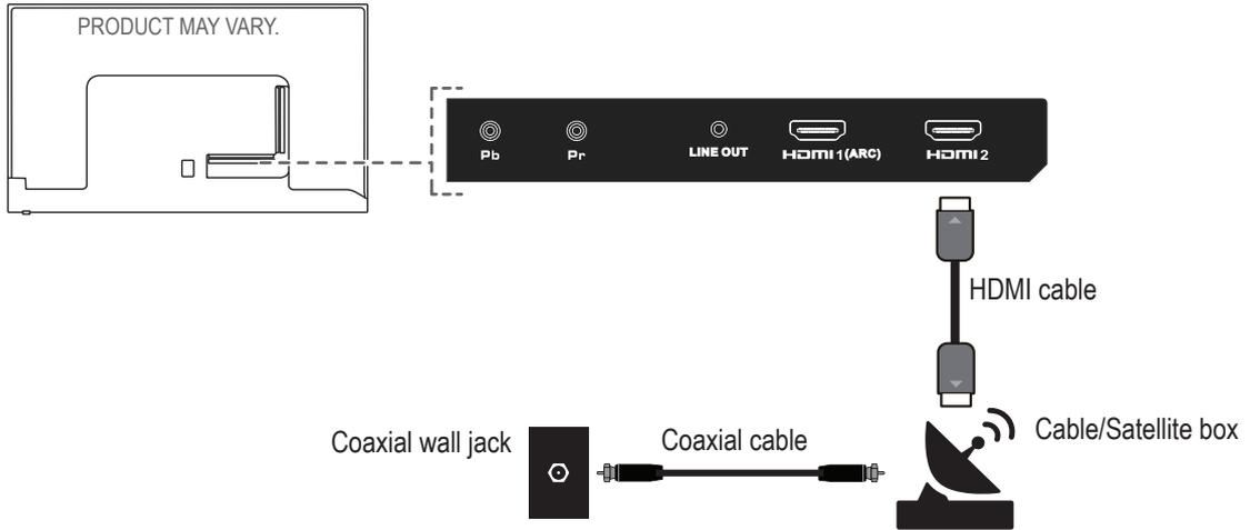
1. Connect an HDMI cable (not included) to the HDMI OUT port on your cable/satellite box.
