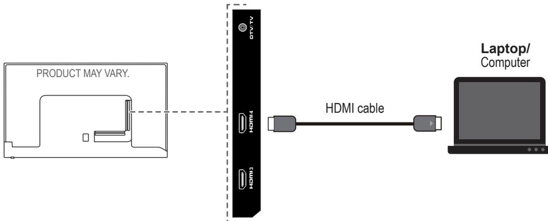
1. Connect an HDMI cable (not included) to the HDMI OUT port on your laptop/computer.
