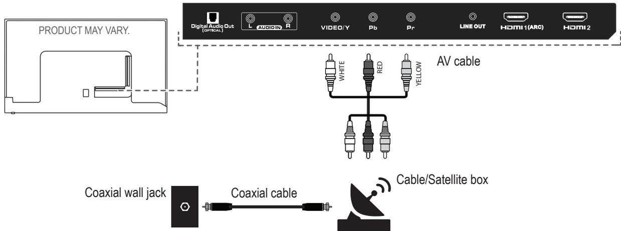
1. Connect an AV (composite) cable (not included) to the AV jacks on your cable/satellite box.
