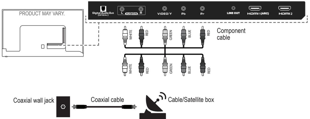
1. Connect a component cable's (not included) red, blue, and green connectors to your cable/satellite box.
